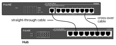
Figure 2-10 Connecting a hub without an uplink port to the Switch
